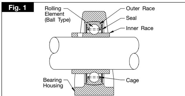
Cool, quiet, and low friction operation requires highly polished surfaces on the rolling elements and races. High load ratings and long bearing life make the use of high strength, high quality steels necessary. Race construction is hardened steel or sometimes alloy steel with just the bearing path hardened. Cage construction can be either plastic, brass, or steel.
