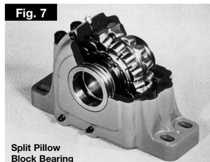
are used in fixed and expansion (sometimes called “float”) combinations. Aerovent uses a fixed bearing for the bearing that is closest to the drive and an expansion bearing for the other one. This arrangement guarantees there is adequate radial load in order to carry the thrust load and guarantees that the rollers will roll properly.
