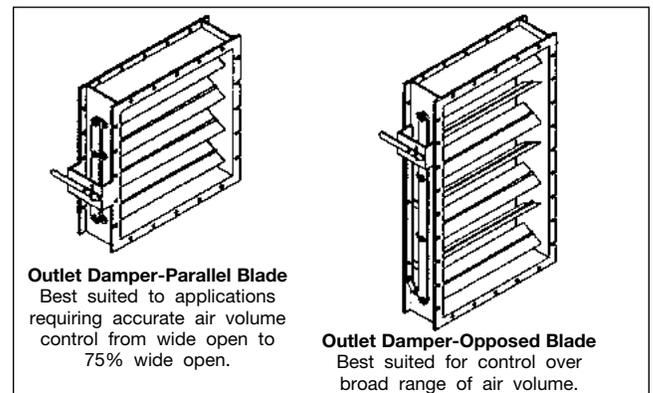
They can be mounted horizontally as shown, with the blades parallel to the fan shaft, or they can be mounted with the blades perpendicular to the fan shaft. Perpendicular blade orientation may require special bearing considerations.
