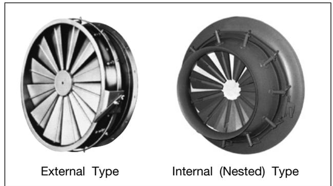
both a resistance and flow modifying effect by pre-spinning the air before it enters the fan wheel, generating a new performance curve for each vane position. The performance curve reacts very similar to a fan equipped with speed control.
