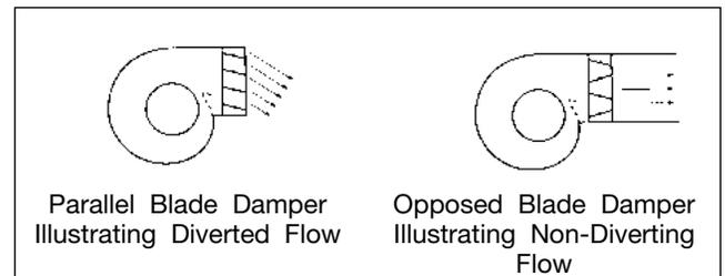
“Opposed” blade dampers are the preferred selection when it is necessary to maintain an even distribution of airflow immediately downstream of the dampers. The airflow characteristics of both the “parallel” blade and the “opposed” blade dampers are illustrated in Figure 6.
