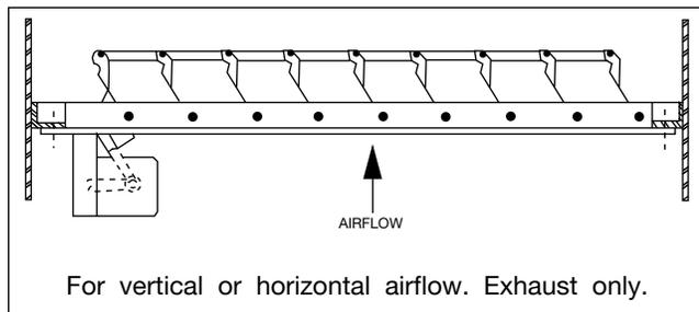
Another advantage of the motor operated damper is that when power is off the spring return insures positive closing of the blades and is not influenced by stray eddies or air currents.
