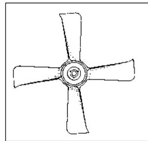
Figure 6. Medium Width Stamped Steel Impeller
