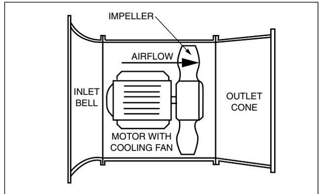
peratures up to 600°F, or air heavily contaminated with corrosive chemicals or explosive vapors. They can be mounted in parallel for higher airflows or they can be staged in series to increase their pressure capabilities. Also, as mentioned under the panel fans, using larger hub-to-tip ratio impellers increases the tubeaxial fan's ability to work against pressure for a given speed or conversely enables the fan to work against the same pressure at a lower speed.
