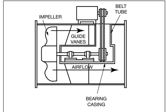
sions. The adjustable pitch versions are limited to clean air applications; however, fans with cast solid impellers can be designed to handle high temperatures and chemical contaminated air. Vaneaxial fans are not recommended for applications containing abrasives, dust, stringy materials or overspray since buildup on the guide vanes will decrease fan performance.
