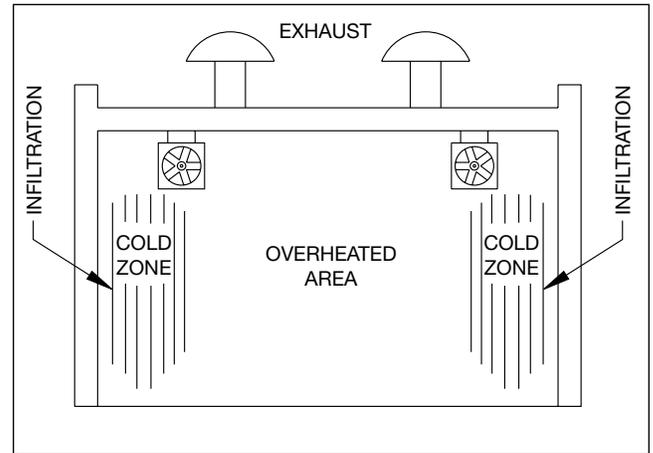
Figure 1 shows how cold zones will occur along walls and overheated zones will show in the middle of the building.
