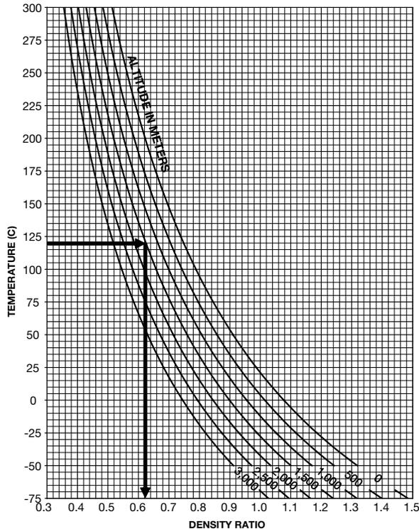
**Example 4:** Select a fan to deliver 4.01 m<sup>3</sup>/s at 0.62 kPa SP at 1,676.4 m elevation at 121.1°C. From Table 1 the factor for 121.1°C is 1.34 and from Table 2 the factor for 1,676.4 m elevation is 1.22. The overall factor is obtained by multiplying these factors: 1.34 x 1.22 = 1.63. To use a fan manufacturer's performance tables, convert the SP to standard air:
