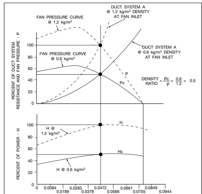
This density ratio must always be considered when selecting a fan from a manufacturer's catalogs or curves.
