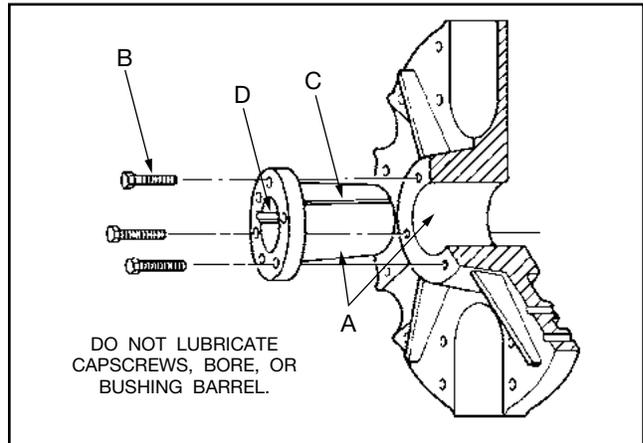
These capscrews force the taper bushing into the hub which in turn compresses the bushing onto the shaft. This makes a positive clamping fit. The torque must not exceed 24 ft. lbs. for Q bushings and for R bushings.
