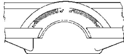
Angle setting index on shank socket. Marked from 10° through 50°. Each mark is 2°. When hub is viewed as shown above, scale on left side should be used for right-hand propeller and scale on right side should be used for left-handed propellers.
