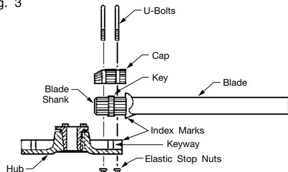
Propellers may be assembled so the cap side of the hub is the inlet side (reverse bore). If blades do not have the index mark on the discharge side, it is then necessary to adjust the blade angle with a protractor.
