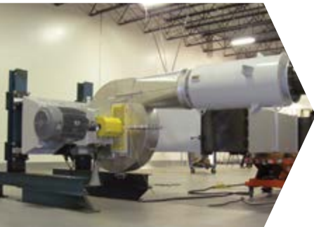
AMCA 210 Air Performance Testing
