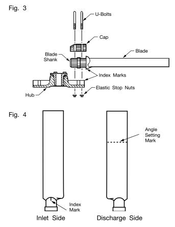
The hub and blades are balanced separately. The weight distribution throughout the length of the blade varies slightly. Therefore, the balance is to a constant moment and blades may be assembled at random even though the weights are slightly different.
