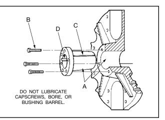
shaft. This makes a positive clamping fit. The torque must not exceed the torque values shown in the chart to the left.
