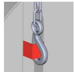
Lifting lugs are provided on most units.
