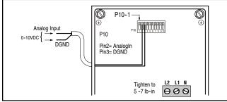
If no speed controller is selected, the motor will be set to run at the nominal motor RPM. Pin 1 will be connected to Pin 2 sending the motor a 10V signal to run at nameplate RPM.
