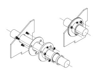
**Theory of Operation** — The sealing action is provided by two lip type seals placed back to front within a seal housing with a layer of grease between them. The grease reservoir may be maintained using the grease fitting in the seal housing. The contact is between the seal inner lip and the circumference of the fan shaft.
