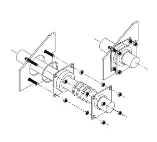
Theory of Operation — The stuffing box is sealed to the fan housing with PTFE joint sealant for a gasketing material. The packing materials are two flexible graphite split rings sandwiched between two carbon yarn anti-extrusion rings. The outside hex nuts force the outside packing plate into the stuffing box, expanding the graphite rings to provide a leak tight seal.
