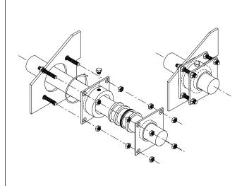
Theory of Operation — The stuffing box is sealed to the fan housing with PTFE joint sealant for a gasketing material. The packing materials are a flexible graphite split ring and a lantern ring sandwiched between two carbon yarn anti-extrusion rings. The outside hex nuts force the outside packing plate into the stuffing box, expanding the graphite rings to provide a leak tight seal. A pressure purge tap is provided to insure that all leakage will be the purge gas.
