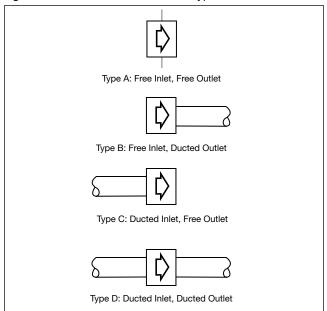
Products that are rated and certified by AMCA must illustrate that they have been rated by one of the installation types shown above.
