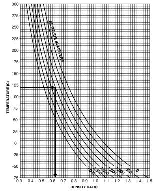
**Example 4:** Select a fan to deliver 4.01 m³/s at 0.62 kPa SP at 1,676.4 m elevation at 121.1°C. From Table 1 the factor for 121.1°C is 1.34 and from Table 2 the factor for 1,676.4 m elevation is 1.22. The overall factor is obtained by multiplying these factors: 1.34 x 1.22 = 1.63. To use a fan manufacturer's performance tables, convert the SP to standard air:
