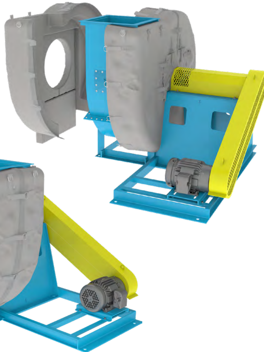
High Temp Applications use a Cooler Box. Insulated Jacket wraps around cooler box.
