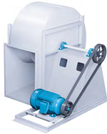
Arrangement 9F Belt Driven Extended Structural Frame to Mount Motor Not suitable for spring isolators
