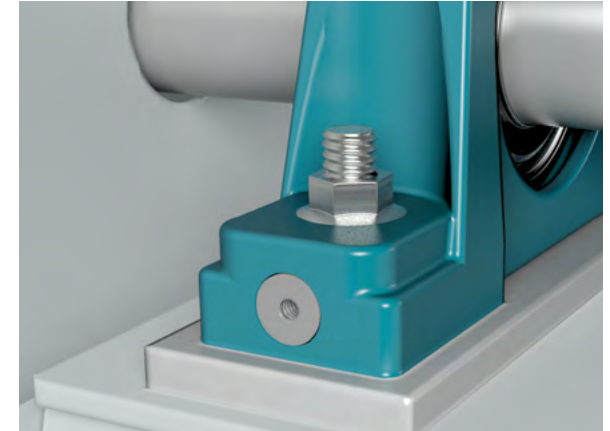
ACCELEROMETER HOLES Drill & Tap: 1/4" - 28UNF with 1" Spot Face Optional: Drill & Tap: 1/4" - 18NPT with 1" Spot Face
