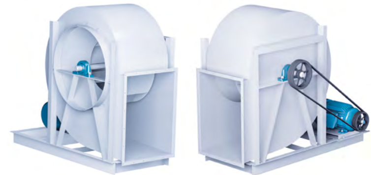
Arrangement 3E Belt Driven Extended Angle Frame to Mount Motor (Fan welded to frame/base - typically not suitable for spring isolators)
