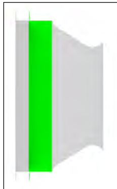
"Green" Section is Added To Extend The Inlet Funnel
