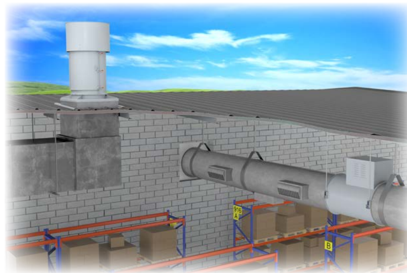
Warehouse Application with VRM & HCH Fans
