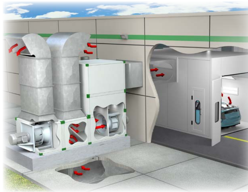
Paint Booth Ventilation
